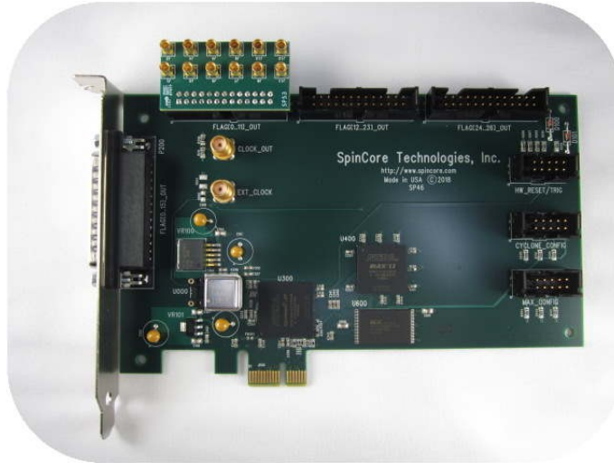
Figure 20: SP53, MMCX Adapter Board orientation and configuration with PulseBlaster SP46 Board.
