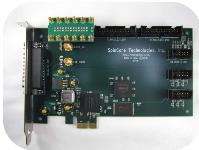
Figure 19: SP32, MMCX Adapter Board orientation and configuration with PulseBlaster SP46 Board.
