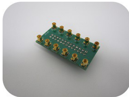
Figure 17: SP32 MMCX Adapter Board allows easy access to individual bits.
