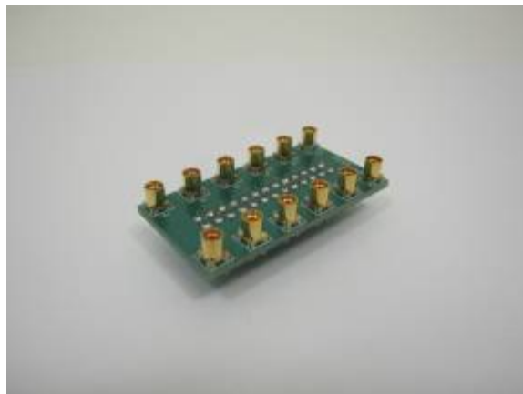
Figure 17: MMCX Adapter Board allows easy access to individual bits.
