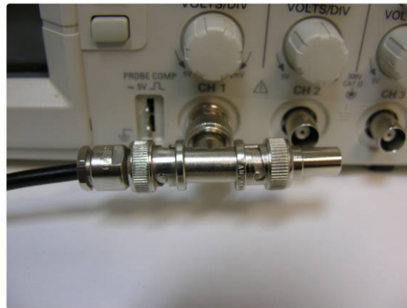
Figure 3: BNC T-Adapter on the oscilloscope input channel with coaxial transmission line connected on the left and BNC 50 Ohm resistor connected to the right to terminate the line.
