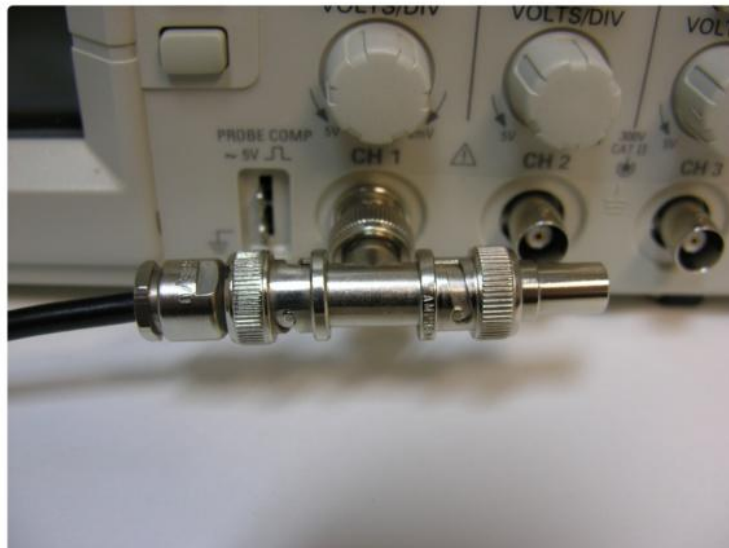
Figure 31: BNC T-Adapter on the oscilloscope with coaxial transmission line connected on the left and BNC 50 Ohm resistor connected on the right, to terminate the line.
