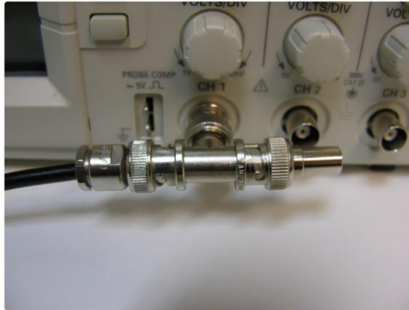
Figure 4: BNC T-Adapter on oscilloscope with coaxial transmission line connected on the left and BNC 50 Ohm resistor connected on the right, to terminate the line.
