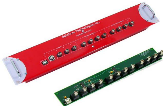
Figure 13: TTL Line Driver assures TTL levels over 50 Ohm loads.
