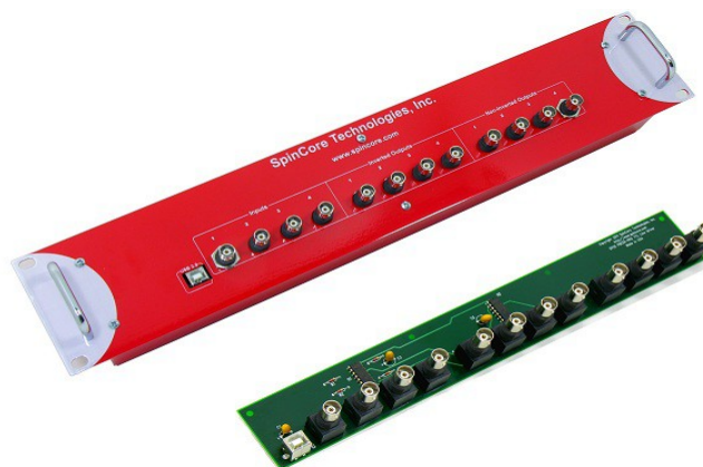
Figure 16: TTL Line Driver assures TTL levels over 50 Ohm loads.
