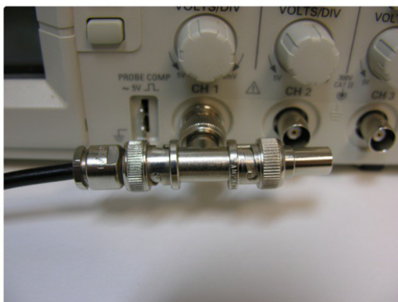
Figure 9: BNC T-Adapter on the oscilloscope with coaxial transmission line connected on the left and BNC 50 Ohm resistor connected on the right, to terminate the line.
