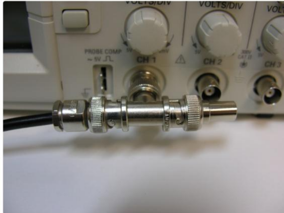
Figure 5: BNC T-Adapter on oscilloscope with coaxial transmission line connected on the left and BNC 50 Ohm resistor connected on the right, to terminate the line.
