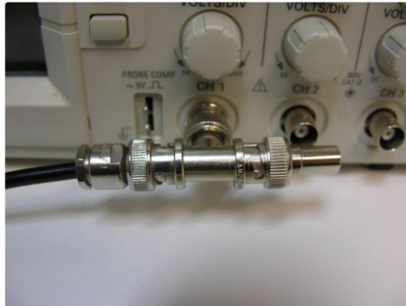
Figure 6: BNC T-Adapter on the oscilloscope with coaxial transmission line connected on the left and BNC 50 Ohm resistor connected on the right, to terminate the line.
