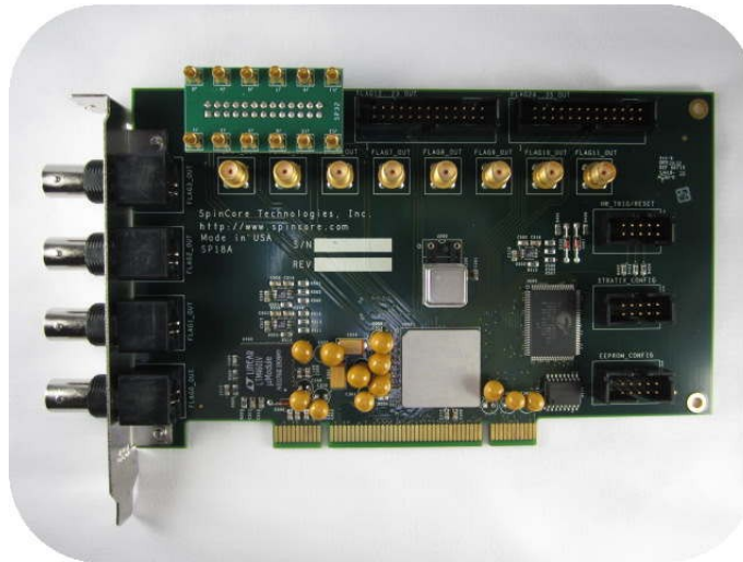
Figure 22: SP32, MMCX Adapter Board orientation and configuration with PulseBlaster SP18A Board.
