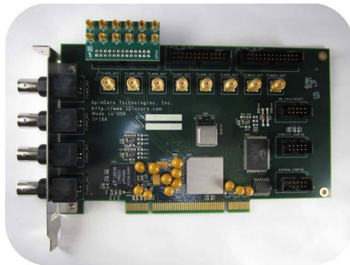
Figure 23: SP53, MMCX Adapter Board orientation and configuration with PulseBlaster SP18A Board.
