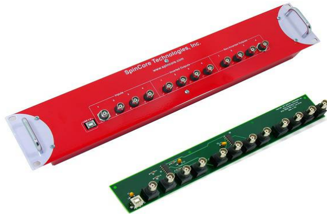
Figure 26: TTL Line Driver assures TTL levels over 50 Ohm loads.
