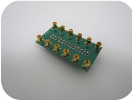
Figure 20: SP32 MMCX Adapter Board allows easy access to individual bits.
