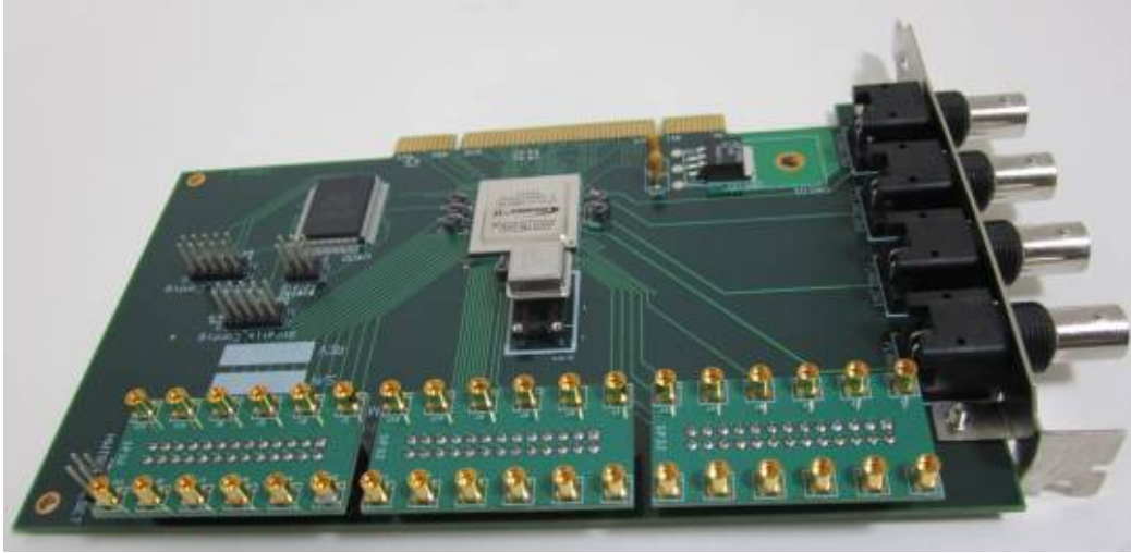
Figure 22: MMCX Adapter Board allows easy access to individual bits.
