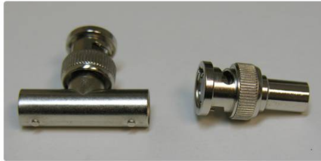
Figure 6: Left: BNC T-Adapter and Right: BNC 50 Ohm resistor.
