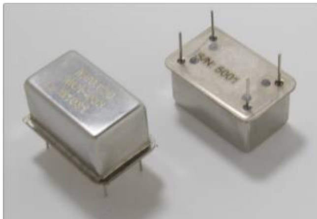
Figure 20: An Oven Controlled Clock Oscillator (or OCXO) with sub-ppm frequency stability is available for the PulseBlasterESR-PRO upon request.
