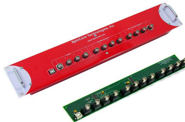
Figure 25: TTL Line Driver assures TTL levels over 50 Ohm loads.
