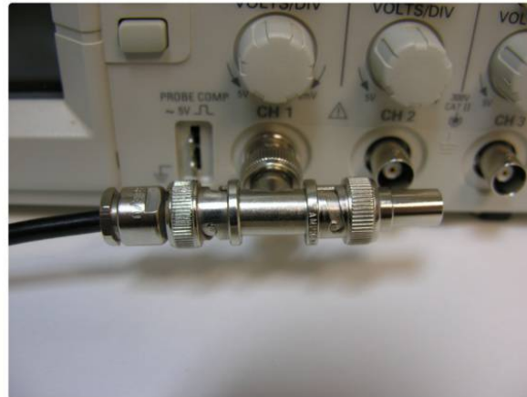
Figure 7: BNC T-Adapter on the oscilloscope with coaxial transmission line connected on the left and BNC 50 Ohm resistor connected on the right, to terminate the line.
