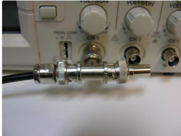
Figure 7: BNC T-Adapter on oscilloscope with coaxial transmission line connected on the left and BNC 50 Ω resistor connected on the right, to terminate the line.
