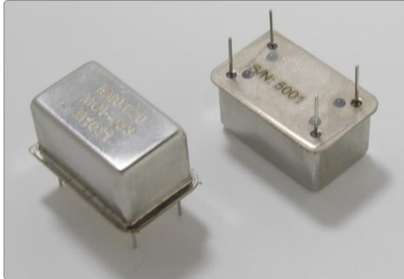
Figure 17: An Oven Controlled Clock Oscillator (or OCXO) with sub-ppm frequency stability is available for the PulseBlaster upon request.
