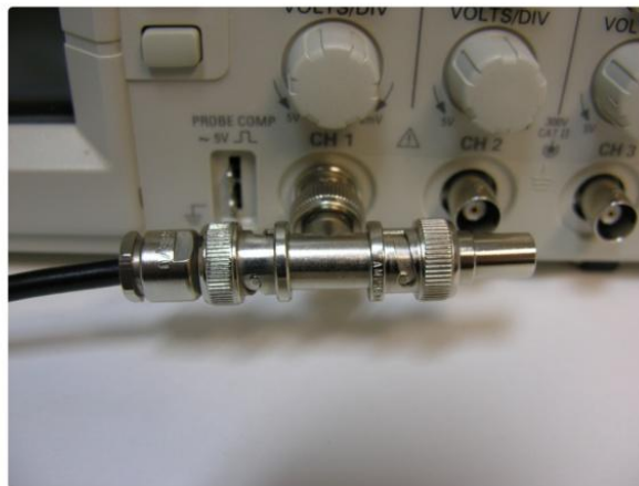
Figure 9: BNC T-Connector on oscilloscope with coaxial transmission line connected on the left and BNC 50 Ohm resistor connected on the right, to terminate the line.
