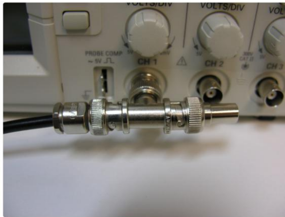
Figure 3: BNC T-Adapter on the oscilloscope with coaxial transmission line connected on the left and BNC 50 Ohm resistor connected on the right, to terminate the line.
