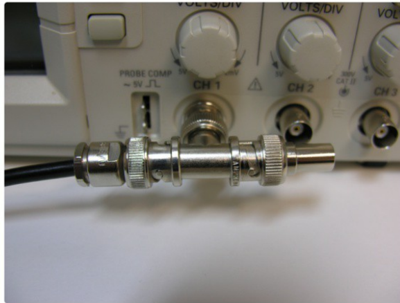
Figure 3: BNC T-Adapter on the oscilloscope with coaxial transmission line connected on the left and BNC 50 Ohm resistor connected on the right, to terminate the line.
