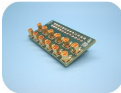
Figure 16: SP53, MMCX Adapter Board allows easy access to individual bits.
