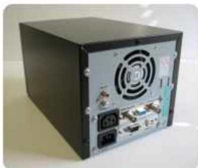
Figure 8. PA15W RF power amplifier – enclosed in a dual-bay enclosure.
