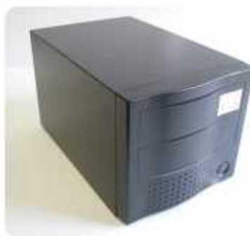
Figure 8. PA15W RF power amplifier – enclosed in a dual-bay enclosure.
