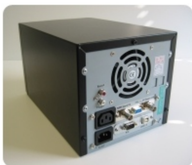
Figure 8. PA15W RF power amplifier – enclosed with iSpin-NMR system.
