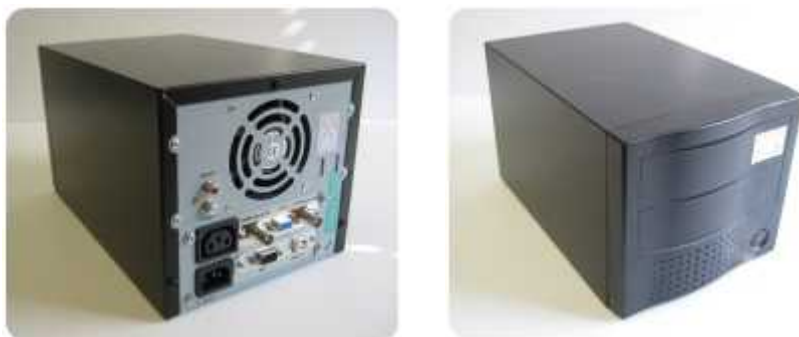
Figure 7: PA15W RF power amplifier – enclosed in a dual-bay enclosure.
