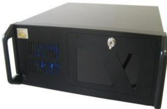
Figure 10: PA100W RF power amplifier – rack-mount enclosure with integrated power supply
