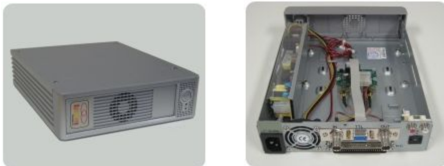
Figure 6: PA10W RF power amplifier – single bay enclosure.
