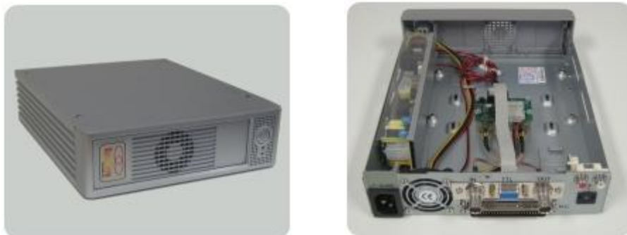
Figure 6: PA10W RF power amplifier – single bay enclosure.
