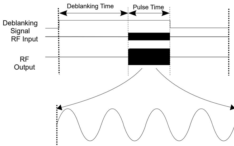
*Figure 4: The RF output has a rise time of approximately 1.5  $\mu$ s until full output power is achieved. A deblanking signal is needed to trigger the RF pulse, and no deblanking interval is needed. The timing in the diagram is exaggerated to illustrate the deblanking signal. NOTE: when operating the power amplifier the duty-cycle for the deblanking signal should be kept low to avoid damage to the amplifier.*
