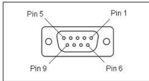
*Figure 6: DB-9 Female Input Connector*
