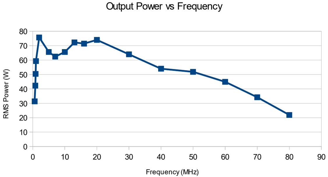
Figure 1: Output Power vs. Frequency of the PA75W RF Power Amplifier.
