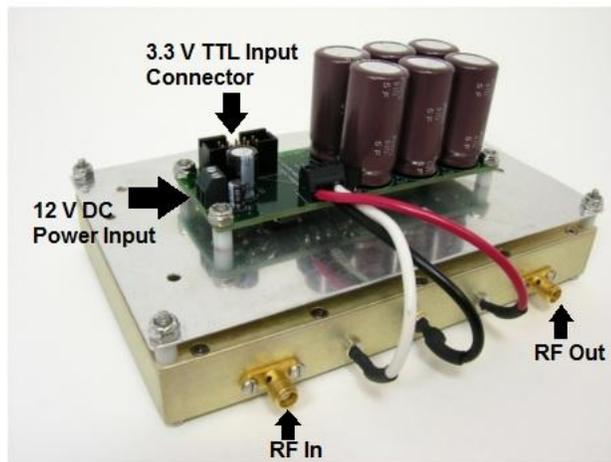
Figure 2: PA75W Connections (Front View)
