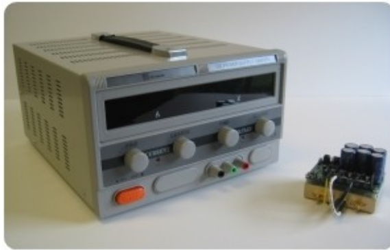
Figure 17: PA100W RF power amplifier – enclosed with DC power supply.
