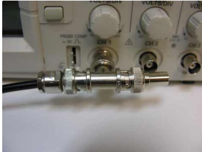
Figure 7: BNC T-Adapter on oscilloscope with coaxial transmission line connected on the left and BNC 50 Ohm Impedance connected on the right, to terminate the line.
