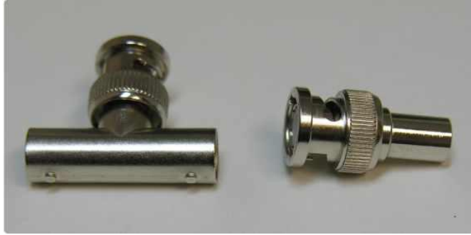
Figure 6: Left: BNC T-Adapter (F M F) and Right: BNC (M) 50 Ohm Impedance.
