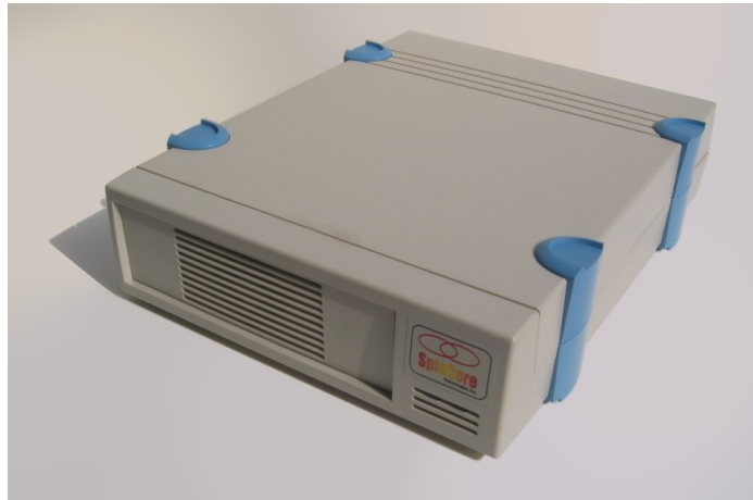
Figure 17: USB RadioProcessor board in a single-bay enclosure.
