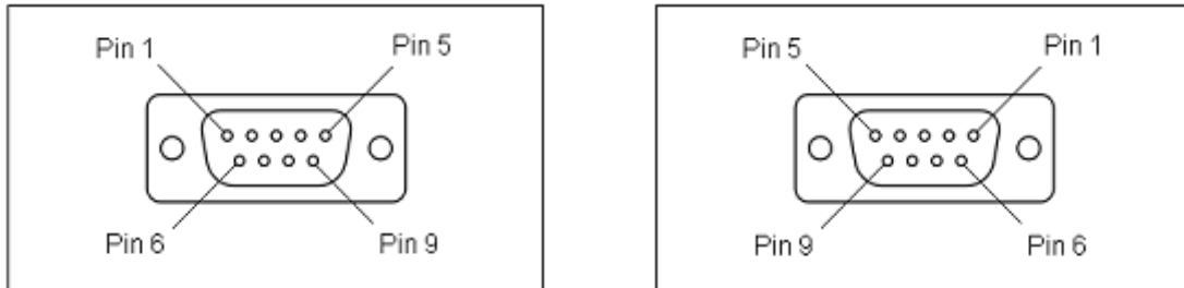
Figure 14: DB-9 Output Connector J300. Left: DB-9 Male. Right: DB-9 Female.
