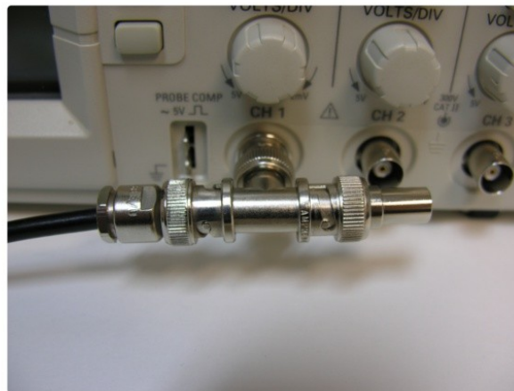
Figure 6: BNC T-Adapter on the oscilloscope with coaxial transmission line connected on the left and BNC 50 Ohm resistor connected on the right, to terminate the line.
