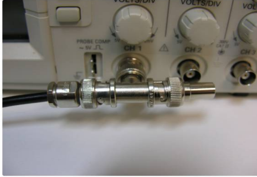
Figure 6: BNC T-Adapter on the oscilloscope with coaxial transmission line connected on the left and BNC 50 \Omega resistor connected on the right to terminate the line.
