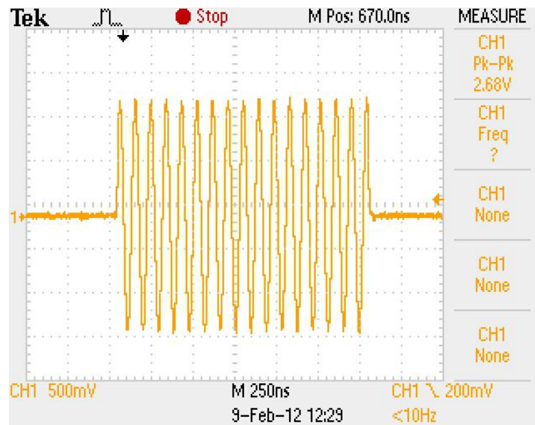
Figure 8: Oscilloscope screen-shot capture of the Spin-NMR Model ETRS transmitter output.
