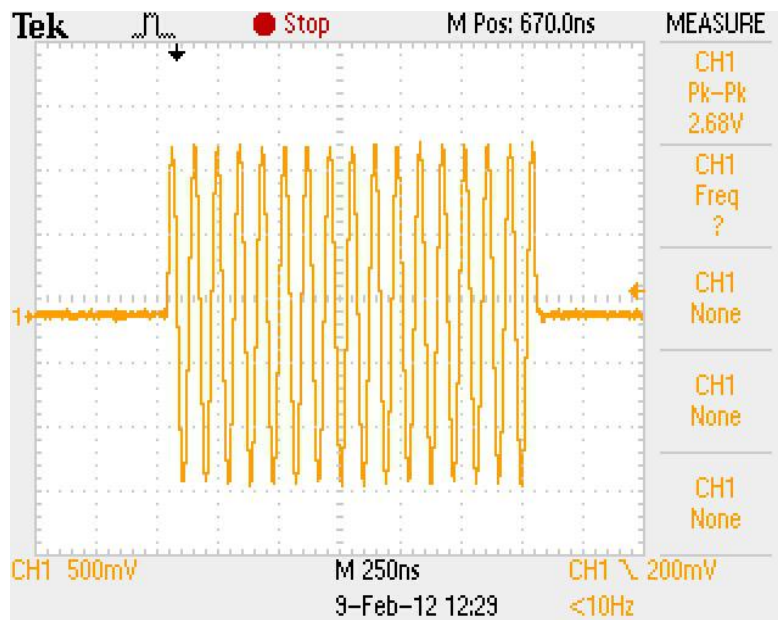
Figure 8: Oscilloscope screen-shot capture of the Spin-NMR Model GX-35 transmitter output.
